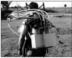
CO<sub>2</sub> Backpack Sprayer Photograph Courtesy of R & D Sprayers
